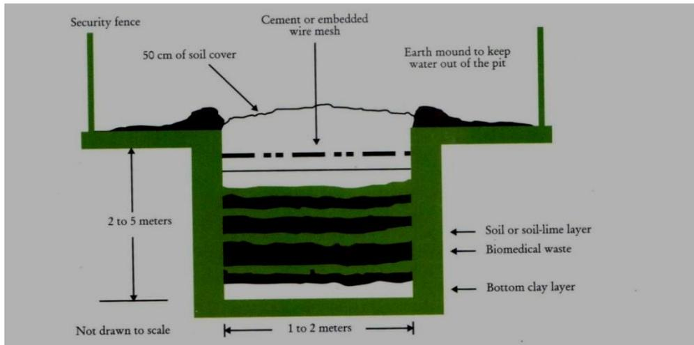
Figure: Layout Specifications for Burial Pit
